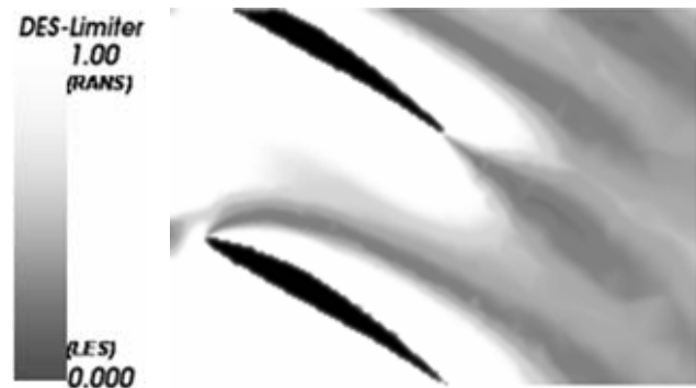
Figure 2: Model mode for the flow in a blade row, with the shielding, proposed by MENTER AND KUNTZ [8]
